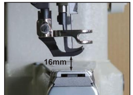
抬壓腳間隙 (16mm)
